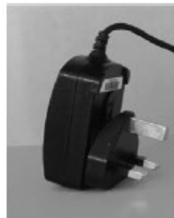
original charging plug 1 A, 5 V
