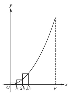
The area A of the region enclosed by the curve, the x-axis and the line x = p is given approximately by the sum S of the areas of n rectangles, each of width h, where h is small and nh = p. The first three such rectangles are shown in the diagram.
