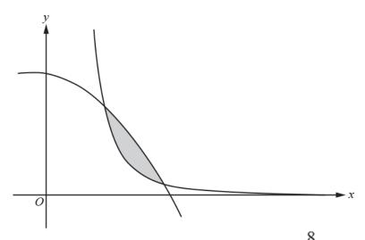
The diagram shows parts of the curves  $y = 11 - x - 2x^2$  and  $y = \frac{3}{x^3}$ . The curves intersect at (1, 8) and (2, 1).
