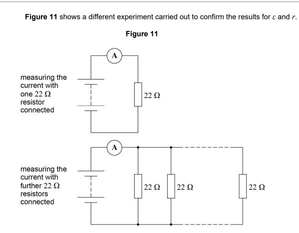
Initially the power supply is connected in series with an ammeter and a 22  $\Omega$  resistor. The current *I* in the circuit is measured.
