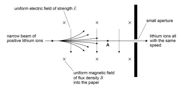
A narrow beam consists of positive lithium ions travelling at different speeds. The beam enters a region where there is an electric field and a magnetic field. The directions of the uniform electric field of strength E and the uniform magnetic field of flux density B are shown on **Figure 3**.
