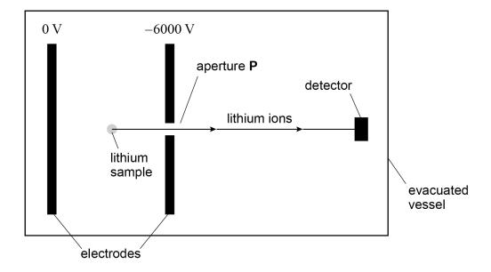
A stationary  ${}^7_3Li^+$  ion in the lithium sample is at the mid-point between the parallel electrodes. The  ${}^7_3Li^+$  ion accelerates towards aperture **P**.
