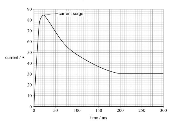
0 4 . 1 Determine the total energy input by the 24 V battery to the motor in the first 200 ms. [3 marks]
