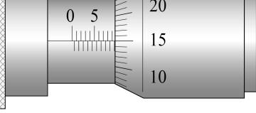
main scale and micrometer scale shown enlarged
