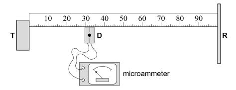
The student places a microwave detector **D** approximately one-third of the distance from **T** to **R**. When **T** is switched off, the microammeter connected to **D** reads zero.
