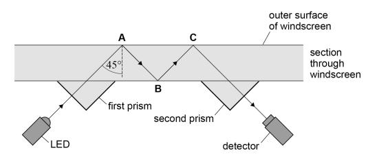
A light ray travels from the light-emitting diode (LED) through the first prism and into the windscreen. The ray reflects off the surfaces of the windscreen at **A**, **B** and **C** and then passes through the second prism into the detector.
