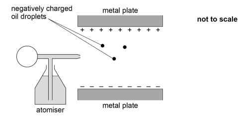
Negatively charged oil droplets are sprayed from the atomiser into the gap between the two horizontal metal plates. A potential difference is applied between the metal plates.
