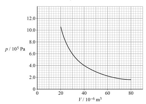
The combustion chamber has a volume of  $20\times10^{-6}~m^3$  and the piston moves through a volume of  $60\times10^{-6}~m^3.$
