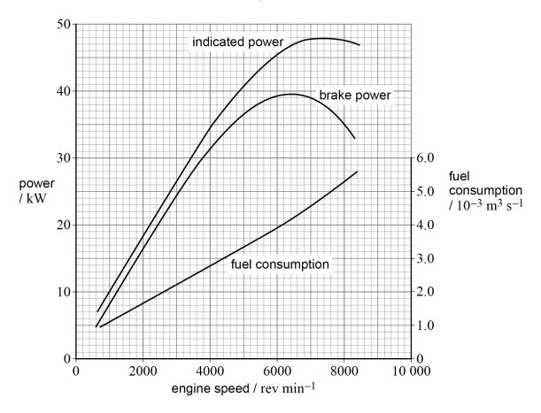
**Figure 4** shows how the indicated power, brake (or output) power and fuel consumption of the engine vary with the engine speed. The scale on the left-hand axis is power and the scale on the right-hand axis is fuel consumption.
