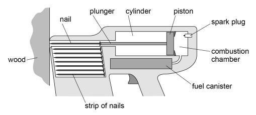
Fuel is mixed with air in the combustion chamber and is ignited by a spark. The gas expands rapidly and drives the piston along the cylinder. The plunger attached to the piston drives the nail into the wood.
