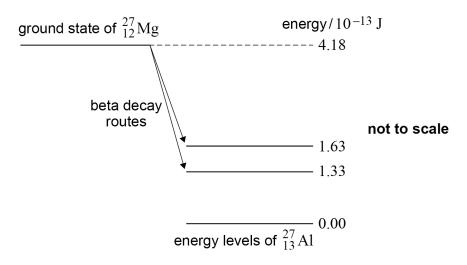
The diagram shows the energy levels and two routes for the beta decay.
