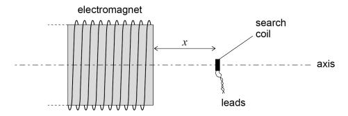
The distance between the search coil and the end of the electromagnet is x. **Figure 8** shows how the magnetic flux density B of the field varies with x.
