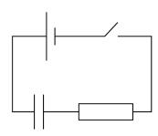
Which pair of graphs shows how the potential difference V across the capacitor and the current I in the circuit change with time t?
