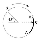
The oven contains an ideal gas kept at a constant temperature. Atoms of the gas emerge from the oven and some pass through the narrow slit **S** in a rapidly rotating drum. The drum is in a vacuum.
