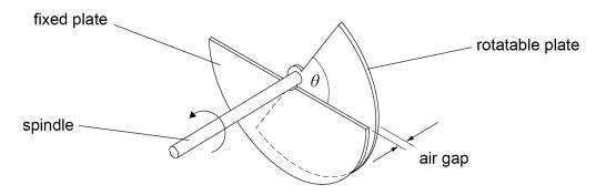
To vary the capacitance, one of the plates is rotated through an angle  $\theta$  using the spindle. The other plate remains fixed.
