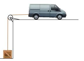
Initially, the van is at rest and the crate rests on the lower level. The rope is taut. The van moves away from the pulley to lift the crate from the lower level. The van's engine produces a constant driving force of 5000 N. A constant resistance force of magnitude 780 N acts on the van. Assume there is no resistance force acting on the crate.
